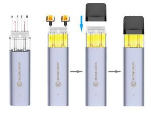
$\boldsymbol{A}$  and  $\boldsymbol{B}$  are the oil filling holes of the left and right tanks respectively.
